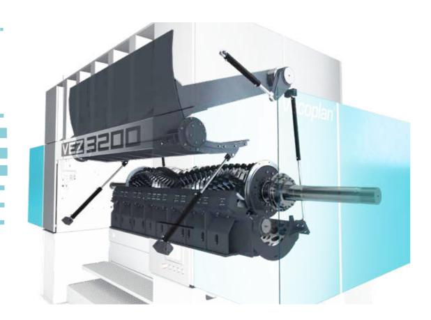
When it gets tough, and large metal parts arise, the tramp material detector takes action and protects the machine. Thanks to the hydraulic base flap, the tramp material is removed in an instant – the machine only stops momentarily. The single-shaft pre shredders offer particularly profitable operation with constantly high throughput and homogeneous output quality.
